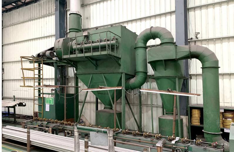
Production plants equipped with dust collectors with filter bags
