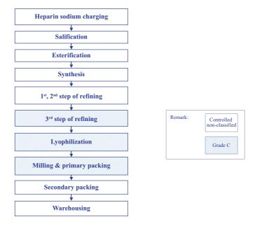
The following diagram summarizes the manufacturing process for our enoxaparin sodium injection in the format of pre-filled syringes:
