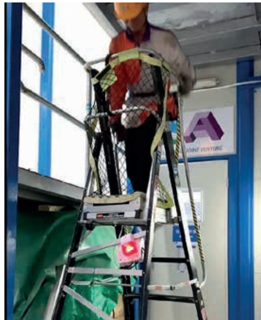
Install a self-developed alarm system on ladder platform to ensure the bottom bracket is completely unfolded and the back railing is fastened when it is in use 在梯台上安裝自行研發之警報系統， 以確保使用時，底部的支架完全伸展 及背後圍欄已扣緊
