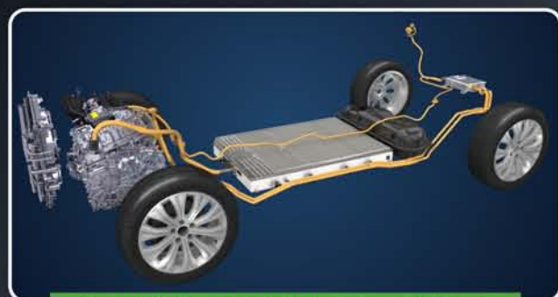
Song PLUS Super Hybrid Chassis Architecture
