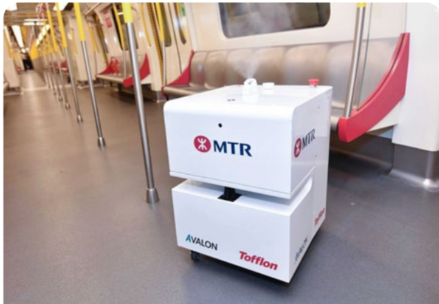
VHP Robot has been deployed to conduct deep cleansing in our trains
