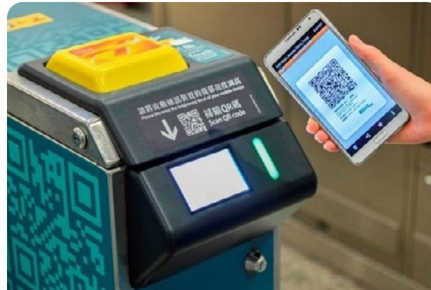
Introducing QR code payment service at heavy rail stations to enable passengers using diversified and flexible payment options
