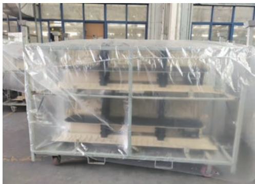
Before the change – with disposable bagging tooling 變更前—帶一次性套袋工裝
