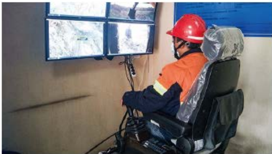
The excavator remotely controlled by the excavator driver through 5G technology is working on the slope of the mining area in an orderly manner
