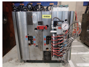
Hot runner mold installed to reduce scrap, saving 25 tons of plastic raw material per year
