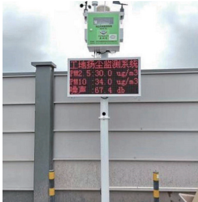
On-site monitoring of dust data 揚塵數據現場監測
