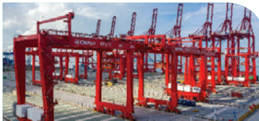
Large port machinery: Successfully developed automation technologies such as the function of automatic grab and release containers, electronic anti-roll, large vehicle anti-collision, trolley/lifting positioning, and the automated terminal project was delivered.
