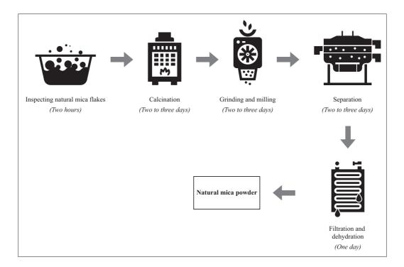
The processing of natural mica flakes into natural mica powder involves the following steps:
