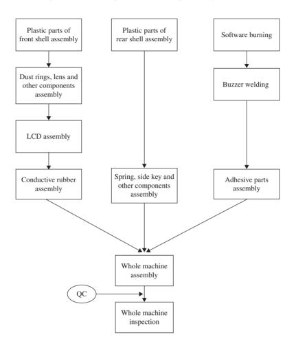
The steps within the dotted line above are conducted in a controlled clean environment (ISO Class 7 or 8), and the other steps are conducted in regular environment. We have implemented quality management systems as part of our manufacturing processes. See "—Quality Control."
