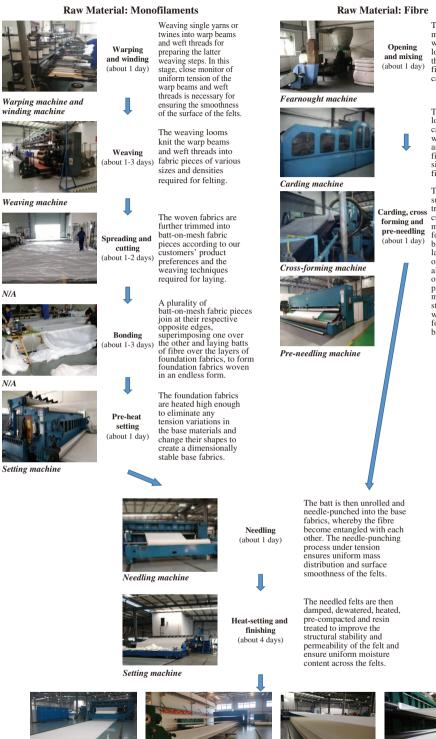
The fibre bale machine is fed with fibre to loosen and mix the lumps of fibres for carding.
