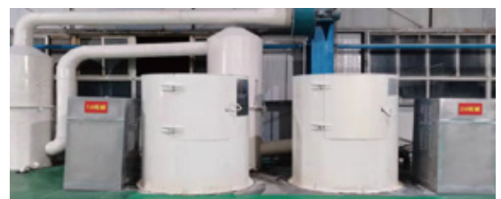
The No. 2 Tungsten Ore Processing Company in China uses a sprinkler system to reclaim dust from the flotation chemicals preparation process. This greatly reduces labor intensity and improves the work environment in the chemicals workshop, reducing exposure to occupational hazards.
