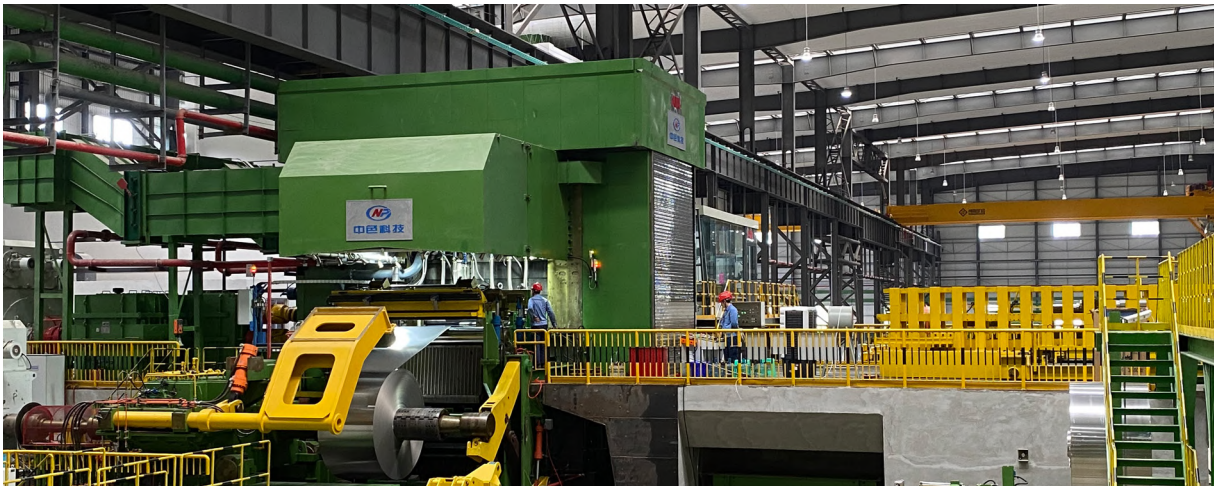
2800mm寬幅鋁板帶冷軋機主機 2800mm wide six-roller aluminum strip cold rolling mill (main body)
