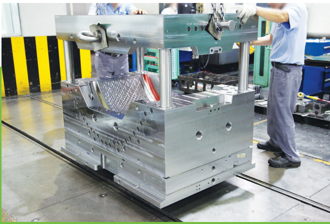
一件大型非標模架正在進行組裝 A large size custom-made mould base is being assembled
