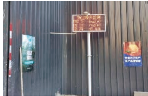
Monitoring over raised dust and noise
