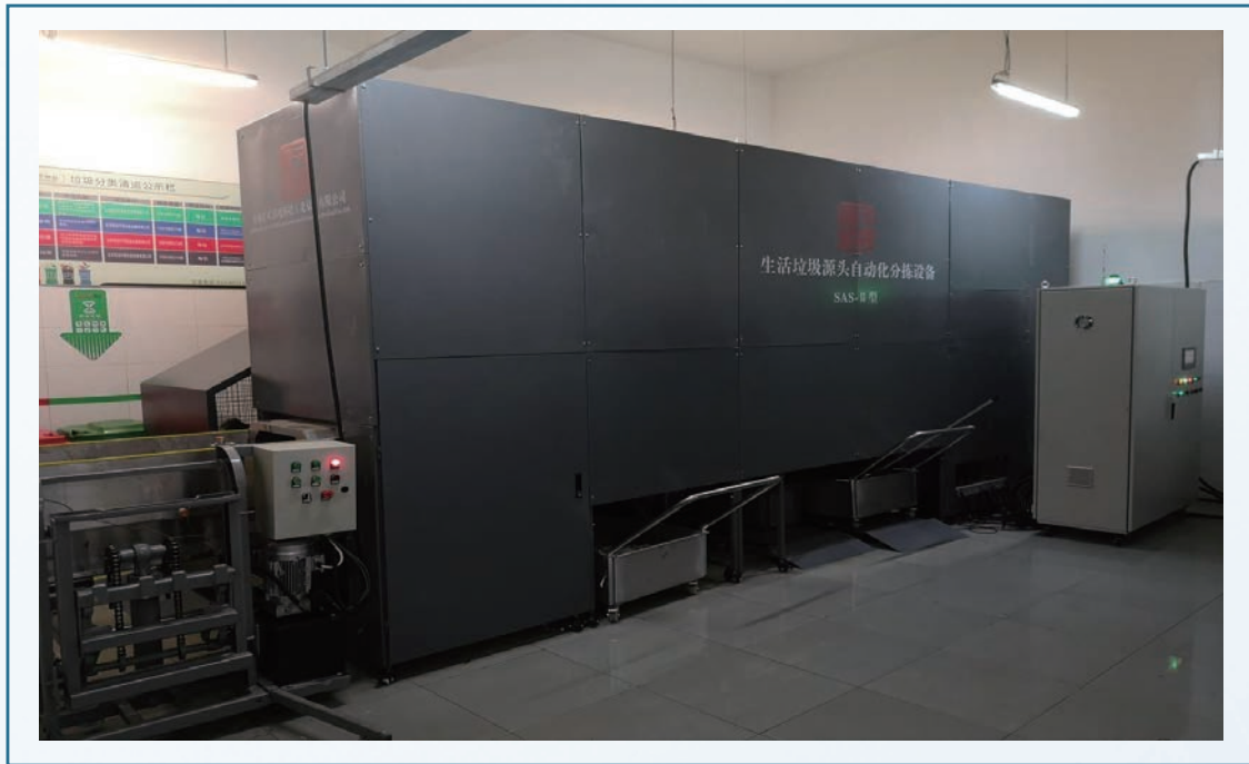
Picture: Intelligent waste sorting equipment
