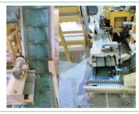
The molding line is equipped with a mud recovery device
