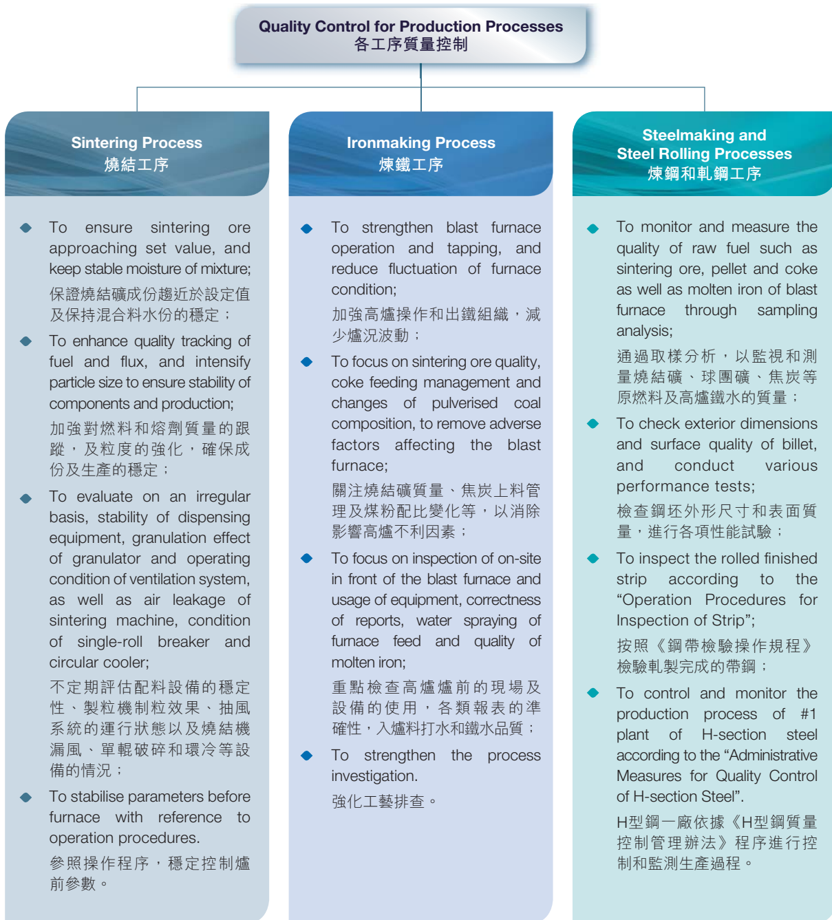
Quality Control for Production Processes of Jinxi Limited 津西鋼鐵各工序質量控制要點
