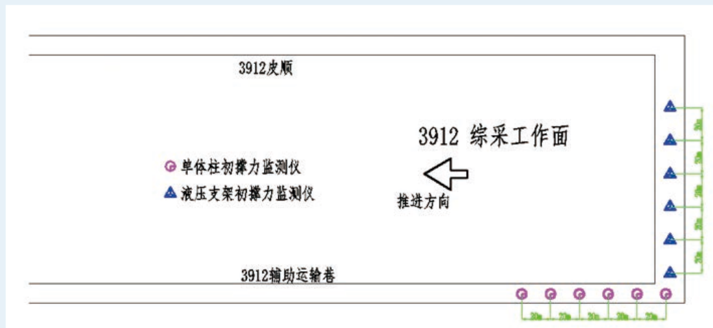
Picture: Single Pillar and Shield Online Pressure Monitoring Layout at Zhaiyadi Coal Mine
