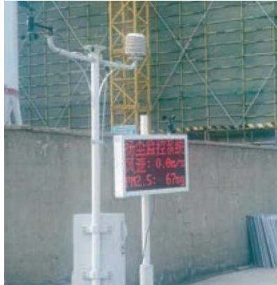
Dust data monitoring 揚塵數據現場監測
