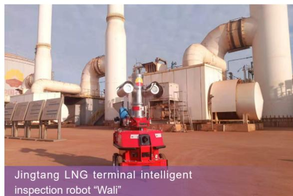
Jingtang LNG terminal intelligent inspection robot "Wali"
