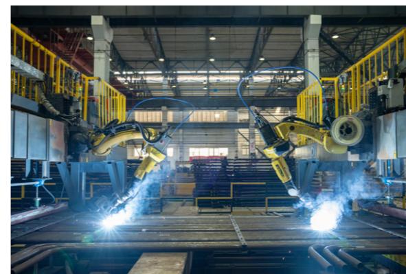
▲ 自主研發蛇形管附件焊接機器人系統、行業首台大型高壓容器全自動鐳射封口焊上線，鍋爐集箱高速數控鑽成功實現「雙機合璧」 The self-developed coiled pipe fitting welding robot system and industry's first full-auto laser sealing and welding machine for large-sized HP vessels form an immaculate pair with high-speed CNC drilling machine for boiler containers
