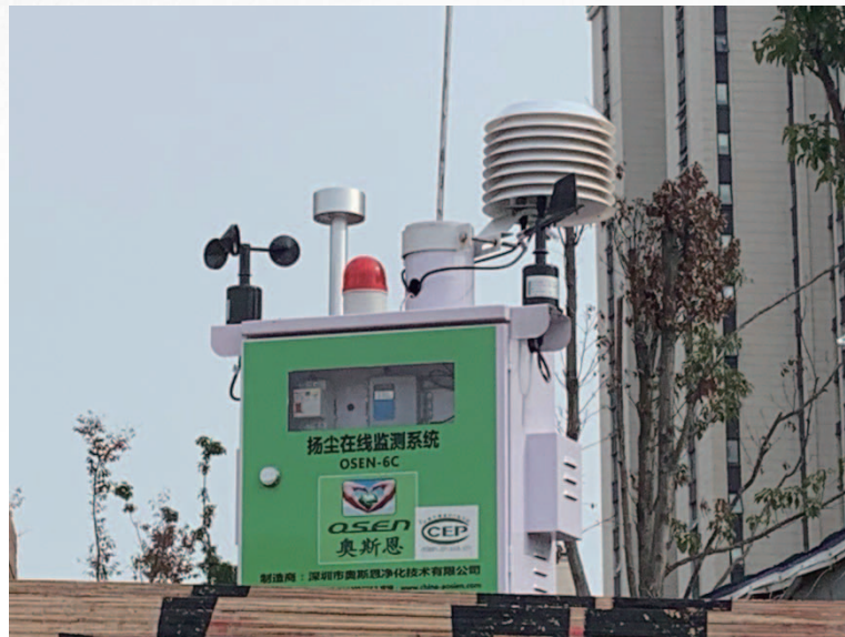
Air quality monitoring system installed on site
