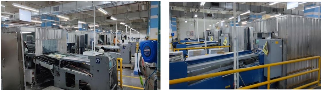
Folding machines with acoustic baffle covers
