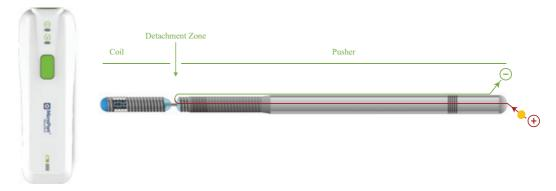
Coil detachment systems commonly employ electrolytic, hydraulic, mechanical or electrothermal mechanisms. *NUMEN FR* utilizes the electrolytic detachment mechanism. The detachment segment disengages when a current is passed through it over time. *NUMEN FR* is classified as a Class III medical device under NMPA regulations and was approved and commercialized in China in July 2020. Together with *NUMEN*, *NUMEN FR* was approved in the United States, the European Union and South Korea in 2021.
