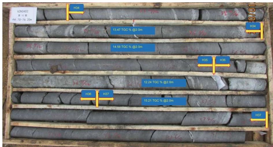
Figure 4–4: Graphitic schist intersected by drillhole VZK0402
