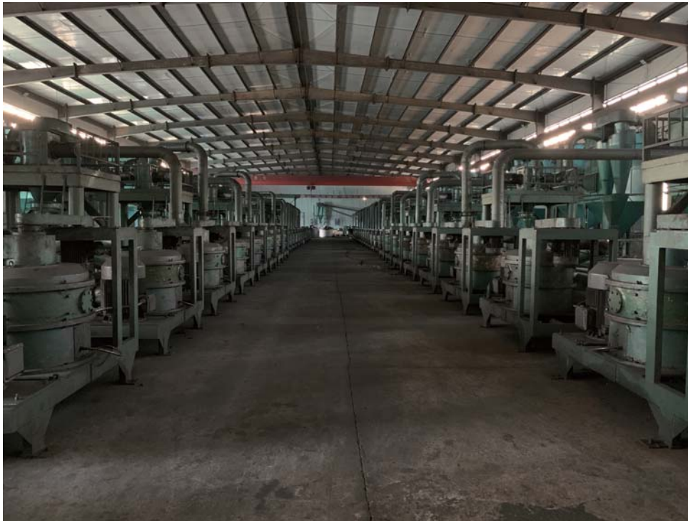
Figure 8–9: Rounding circuit in the spherical graphite processing plant
