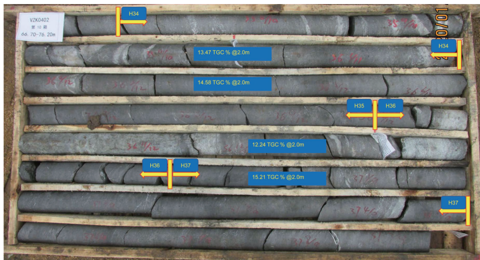
Figure 4–4: Graphitic schist intersected by drillhole VZK0402
