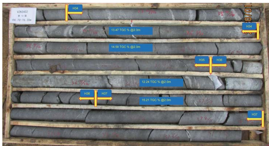
Figure 4–4: Graphitic schist intersected by drillhole VZK0402
