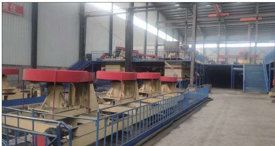
Figure 8–6: New flotation machines
