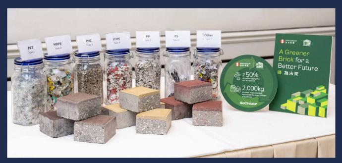
The solution upcycles all seven types of plastic waste, including mixed and composite plastic that are currently impossible to recycle, into sustainable construction materials.
