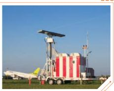
Figure 4: Warning Radar for Bird Strike Prevention
