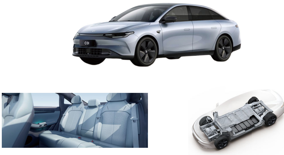
The exterior and interior of the C01 and the CTC structure
