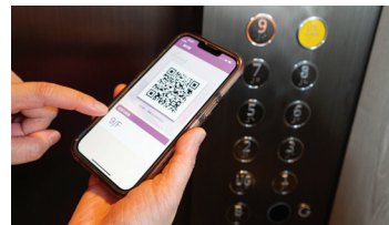
Smart Community app sends out QR code to replace traditional resident cards for owners to enter the main complex gate, lobby doors and controls lifts within the site
