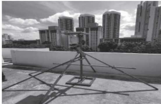
Solar panels used for real time noise monitoring
