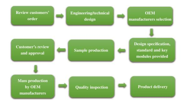
We generally outsource the production of our telecommunication equipment to OEM manufacturers. In addition, we assemble limited number of our IoT antennas with simple design, and perform certain key production procedures that may affect the performance of our IoT antennas, such as soldering, in our assembly and testing center in Shenzhen. Key process of our outsourcing production consists of:
