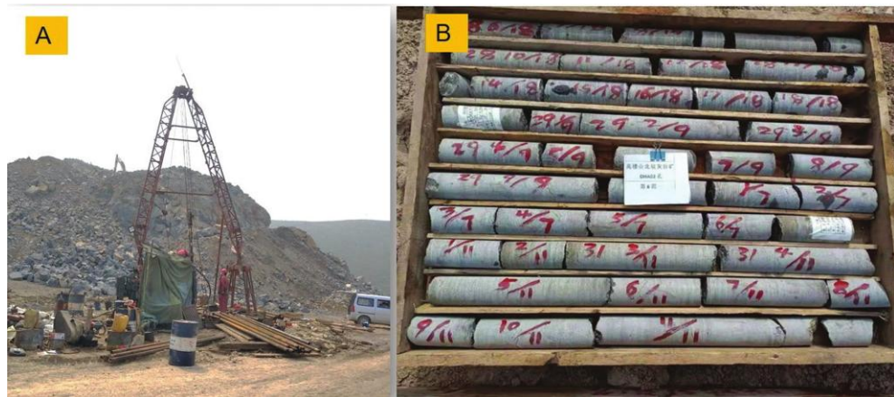
Figure 4-4: Resource definition drilling
