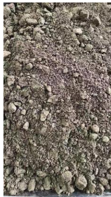
Cement stabilised macadam
