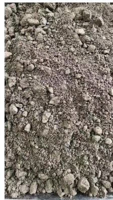
Cement stabilised macadam
