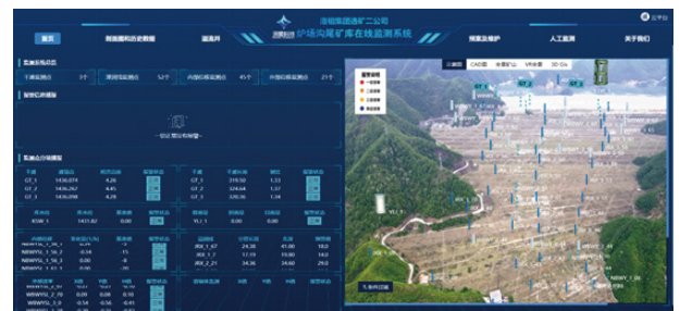
■ In China, key TSF metrics are tracked online in real time to provide early warning of potential hazards.
