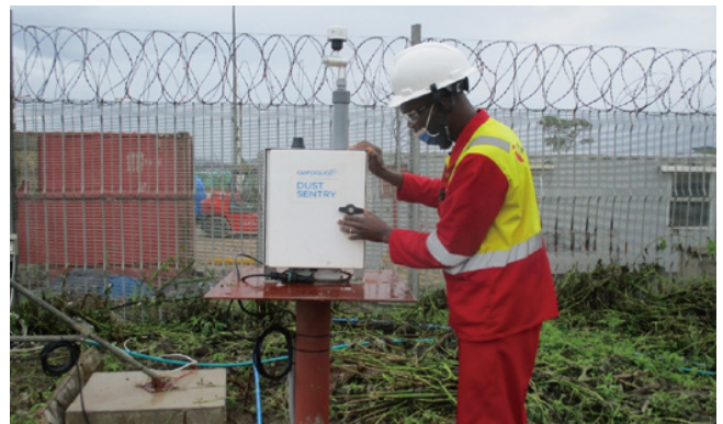
In 2022, TFM upgraded its on-site PM_{10} monitoring equipment to enable automatic, online monitoring in real time.
