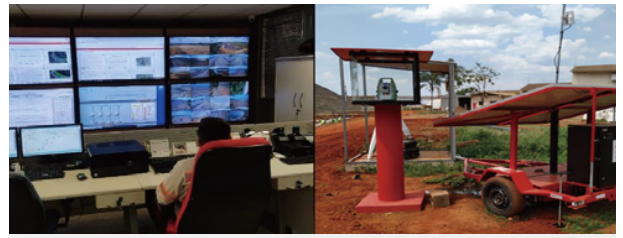
CMOC Brasil installed microseismic monitoring systems at TSFs to enable continuous displacement monitoring.
