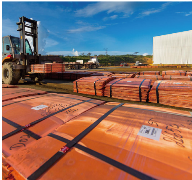
At our TFM site in the DRC, all of our copper and cobalt is labelled with traceability system to enable traceability from the mine to the process plant.
