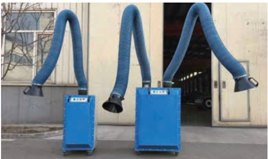
The prefabrication site equipped with mobile welding fume collector and other waste collection and treatment equipment.
