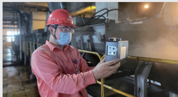
Fuel personnel is measuring the dust concentration after the dry fog dust suppression device is started
