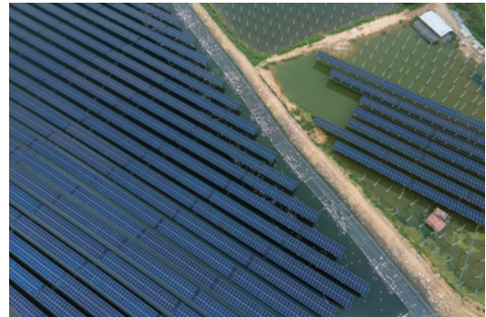
Graph: “Fishery and PV industry complementation” model in Ma'an Community featured “generating electricity above the water and raising fish in the water”, financed by Guangdong Branch of the Bank.
