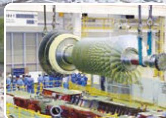
▲ Shop assembly of L10 gas turbine
