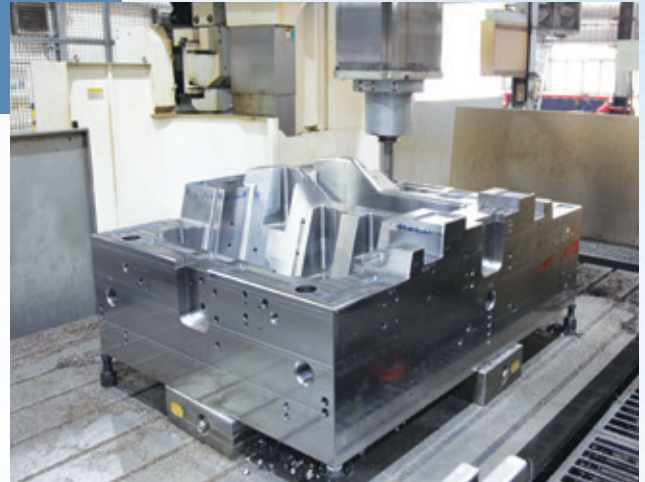
一件大型非標模架正進行加工 A large size custom-made mould base is undergone machining
