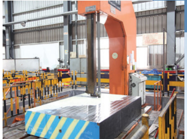
■ 帶鋸正在把大型鋼塊切成粗形 A band saw is cutting a large steel block into rough shape
