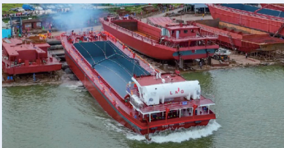
Natural gas fuel supply system with double cold boxes on both sides
