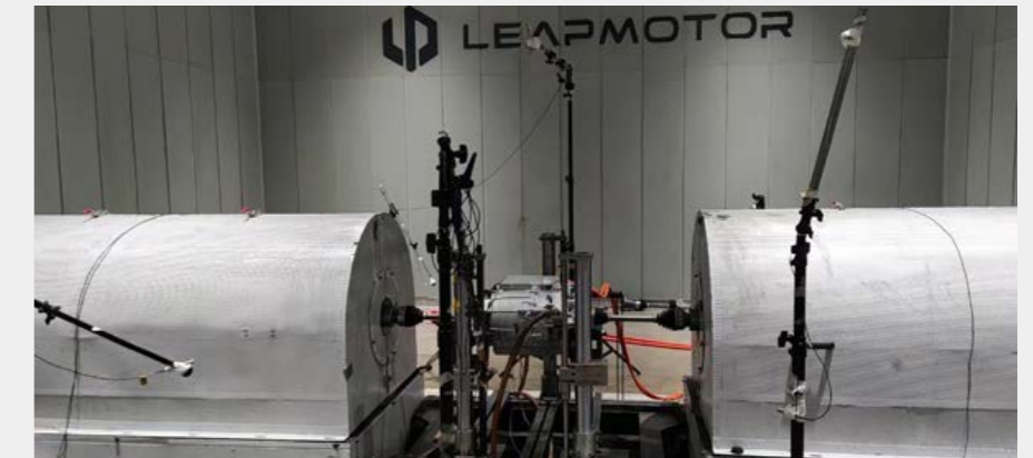
Electric Drive Semi-Anechoic Chamber
