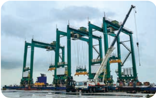
Guangzhou South China Oceangate Terminal and Guangzhou Nansha Stevedoring Terminal completed the transformation of lithium batteries for diesel engines.
