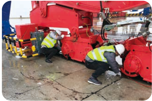
CSP Wuhan Terminal strictly implemented the regulations on safety operation in snowy weather. Before the extreme cold weather came, it conducted a test run on the quay cranes and other machinery, and installed iron wedges to ensure safe operation of the equipment.
