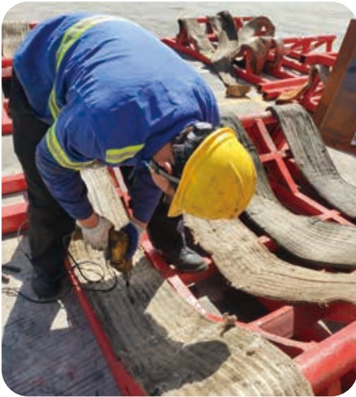
The employees of Jinjiang Pacific Terminal installed scrapped hoisting belts on the saddles of steel coils to recycle the waste in a reasonable way.
