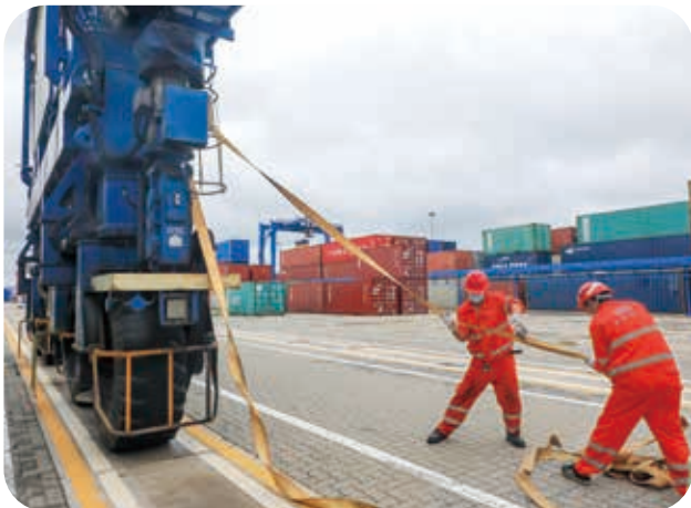
In September 2022, the force 7 gale of typhoon "Muifa" directly affected normal operations. Nantong Tonghai Terminal reinforced the containers in the yard and terminal equipment in accordance with the Company's typhoon preparedness guidelines to ensure the safety of life and property.
