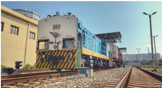
Automated molten iron transportation locomotive
