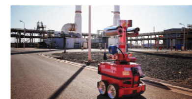
Intelligent inspection robot
